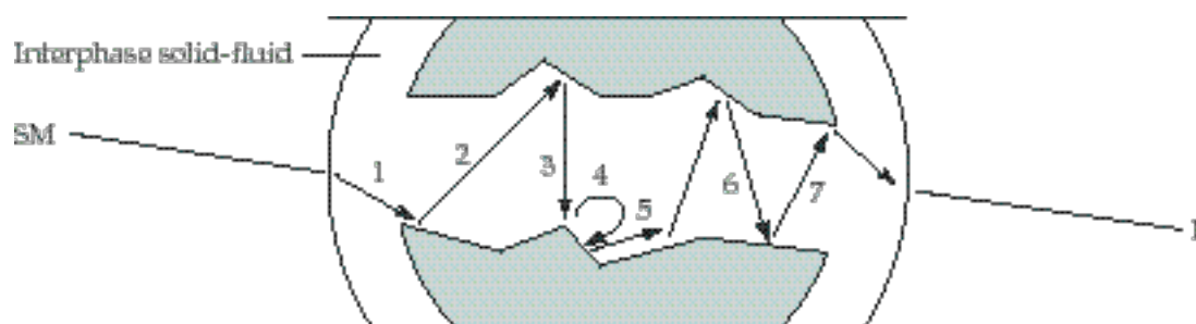
Figure 6 - Reaction steps of a heterogeneous catalytic reaction from SM to P around and inside a catalytic particle with pores of mean diameter d_p . See text for the meaning of numbers 1-7.
